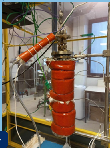
Photo of the pyrolysis system with a reflux zone
