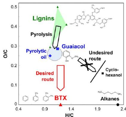
Figure 2: Catalytic pyrolysis of biomass: superior selectivity of hierarchical zeolites to produce aromatic hydrocarbons
