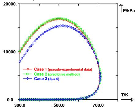
Figure 2: Modelling of a swelling experiment using the PPR78 equation of state
