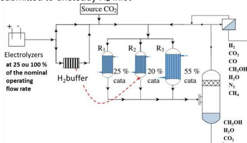
Figure 1: Flow circulations inside a structured heat-exchanger reactor with integrated heat valorization
