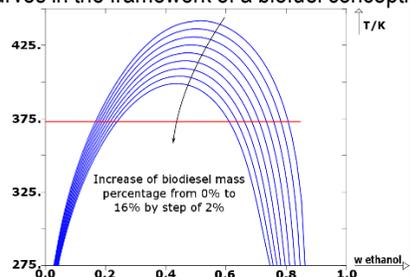
Figure 2: Phase diagram of an 'ideal' working fluid for an absorption demixing heat pump.
